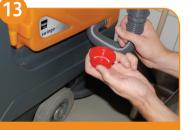
Drain recovery tank with the hose on the side, then drain the solution tank with the hose on the back-side of the machine.
