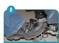
Lower brush unit with foot pedal, then briefly pull the operating lever for brush drive to allow coupling of tool.
