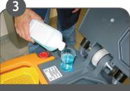
Dose cleaning product into dosing aid, then pour into the grey solution tank.
