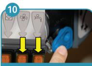
Switch on the solution supply and vacuum motor (left and middle switch).
