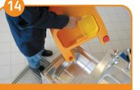
Rinse the recovery tank with fresh water, so it can be removed from the machine.
