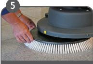
Position tool carefully under the lifted brush unit.
