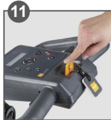
11 Start machine by pushing the key
