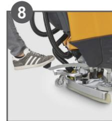
8 Lower brush units by using the manual lever (by foot)
