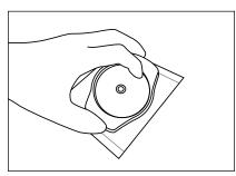
Gently apply pressure on 3M Petrifilm 6 Spreader to distribute inoculum over circular area before gel is formed. Do not twist or slide the spreader. Lift 3M Petrifilm Spreader. Wait a minimum of 1 minute for gel to solidify.
