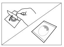
3 Roll the top film down onto the sample to prevent trapping air bubbles. Place the 3M<sup>™</sup> Petrifilm<sup>™</sup> Spreader with the flat side down on the center of the plate. Press gently on the center of spreader to distribute the diluent evenly. Remove the spreader and allow the plates to remain closed for a minimum of 1 hour before use.
