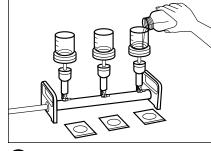
For membrane filtration of water samples use a 47mm, 0.45 micron pore size Mixed Cellulose Ester (MCE) filter.
