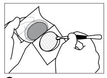
6 Place filter in the center of the hydrated area. Roll top film down to minimize air bubbles or gaps between the filter and the 3M Petrifilm *Enterobacteriaceae* Count Plate.
