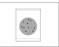
3M Petrifilm Enterobacteriaceae Count Plates can be counted on a standard colony counter or other illuminated magnifier. Colonies may be isolated for further identification. Lift top film and pick the colony from the gel.
