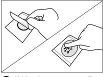
Lightly apply pressure to ensure uniform contact of the filter with the gel and to eliminate any air bubbles.
