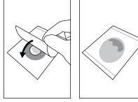
Roll the top film down onto the sample Δ gently to prevent trapping air bubbles. Do not let the top film drop.
