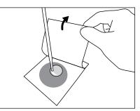
Place the 3M Petrifilm Enterobacteriaceae Count Plate on a level surface. Lift the top film and with the pipette perpendicular to the inoculation area, dispense 1mL of sample suspension onto the center of the bottom film.
