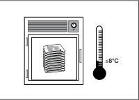
Store the unopened 3M Petrifilm Enterobacteriaceae Count Plate pouches at frozen or refrigerated temperatures lower than or equal to 8°C (46°F). Use before expiration date on package. It is best to allow pouches to reach room temperature before opening.
