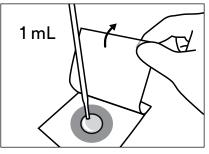
Place 3M Petrifilm Enterobacteriaceae Count Plate on a flat, level surface. Lift the top film and dispense 1 mL of an appropriate sterile hydration diluent onto the center of the bottom film. Appropriate sterile diluents include sterile water, deionized (DI) water and reverse osmosis (RO) water.
