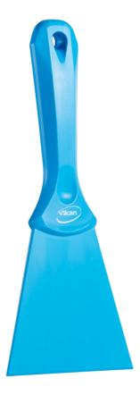
Suitable for loosening stubborn dirt like pastry, chocolate, burnt on food, etc. on smooth surfaces. The nylon blade is a good alternative to a stainless steel blade and can be used on sensitive surfaces to avoid scratches on equipment and sensitive conveyor belts. The hard blade can withstand hot surfaces when used at intervals of max. 2 minutes at a time.
